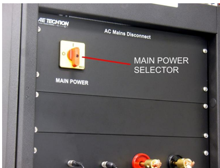
Figure 3.1 Main Power Selector
