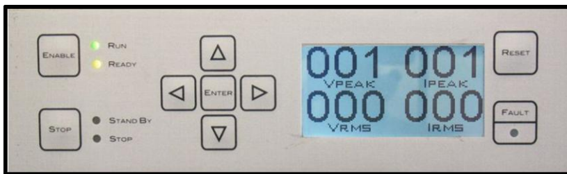
Figure 3.3 Enabled Channel LED Display
