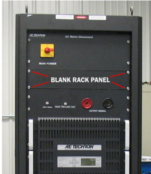
Figure 5.1 Removing the Blank Rack Panel
