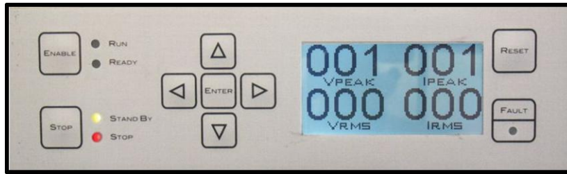
Figure 3.2 Default LCD Screen Display
