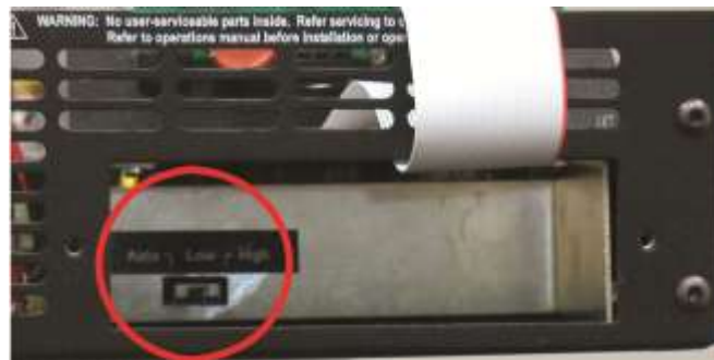
Figure 4.14– Bi-Level Power Switch Location
