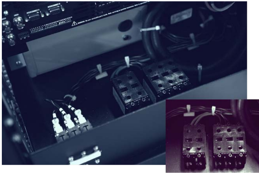
Figure 2.12 – Location of AC Mains Barrier Strip
