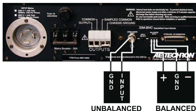
Figure 2.11 – Wiring for unbalanced or balanced input connector
