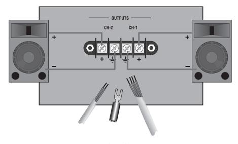
Figure 2.5 Output Connector Wiring
