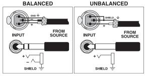
Figure 2.3 Balanced Input Connector Wiring
