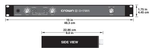
Figure 2.1 D-45 and D-75A Dimensions
