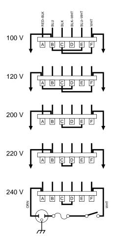
Fig. 2.3 AC Mains Voltage Conversion
