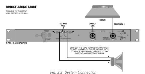
loudspeakers, you can use bridge-mono mode without actually bridging the outputs. Bridge-mono mode is like dual mode except the channel 1 input feeds both outputs, and the channel 2 output is inverted. To use bridge-mono mode without bridging the outputs, wire your loudspeakers as you would for dual mode, <u>but</u> invert the polarity of the channel 2 output wiring (positive goes to negative, and negative goes to positive).
