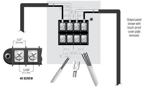
Figure 3.5 Output Connector Wiring (Typical of two channels)
