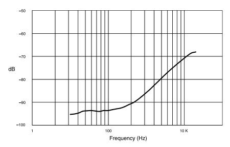
Figure 7.7 CTs 8200 Typical Crosstalk vs. Frequency
