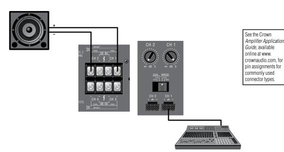
Figure 3.8 System Wiring and Control Settings, Bridge-Mono Mode, 16/8 Ohm.
