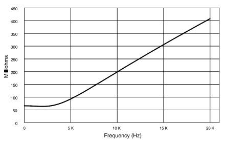
Figure 7.6 CTs 8200 Typical Output Impedance vs. Frequency
