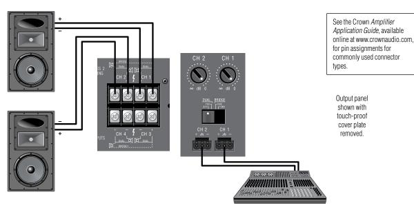
Figure 3.6 System Wiring and Control Settings, Dual Mode, 8/4 Ohm
