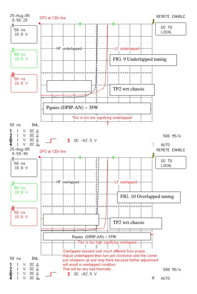
Measuring the real power draw is another good check to determine if the system is adjusted and operating correctly. By using the scope math functions to determine the real power draw based on the mean of RMS line voltage times RMS line current the table below lists approximate power draw value ranges for 3 different operating conditions using each of the 3 DPIP modules:
