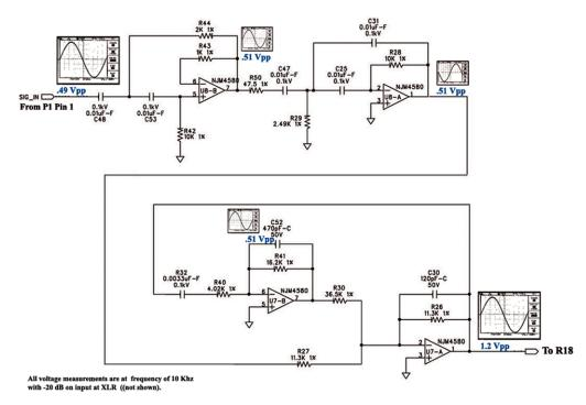
The EON 10G2 utilizes bi-amplification topology to actively filter and separate the high frequency signal from the low frequency signal. Consequently, the low frequency processing circuits are similar. These frequency separation characteristics allow usage of independent, dedicated components for accurate signal reproduction.
