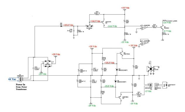
This is the power supply circuit of the EON 10-G2. Operational voltages, necessary of the main amplifier and processing circuits, are created on this PCB. The schematic, shown above, contains three individual circuits: the signal shutdown, the main rectification and low voltage power supply circuits.
