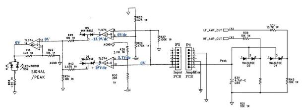
Signal indication is performed by the above circuitry with the possibility of three scenarios--normal ac signal present, no signal present and peak signal present.
