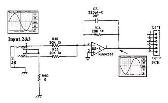
Above is the Tip Ring Sleeve jack input circuitry. The input signals are attenuated by R33 and R46 before reaching isolation IC U5A. Multi-path feedback is used to decrease the distortion and increase the stability of the amplifier. The output signal on pin 1 of U5 connects to pin 5 of connector RC1 where volume control, VR2, (not shown) can control the amplitude delivered to loop/mix summing amplifier, U5B (not shown).
