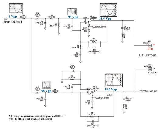
This is the low frequency amplifier. The bridged mode configuration using two LM3886T monolithic amplifiers, U1 and U2, enable twice the output voltage capability than if one IC were driven alone. Therefore, it is strongly recommended this unit be connected to the ac mains through an isolation transformer for safety purposes during the servicing of the amplifier/ output stage. This will separate the grounds from interacting with the test equipment, the unit under test and the technician.
