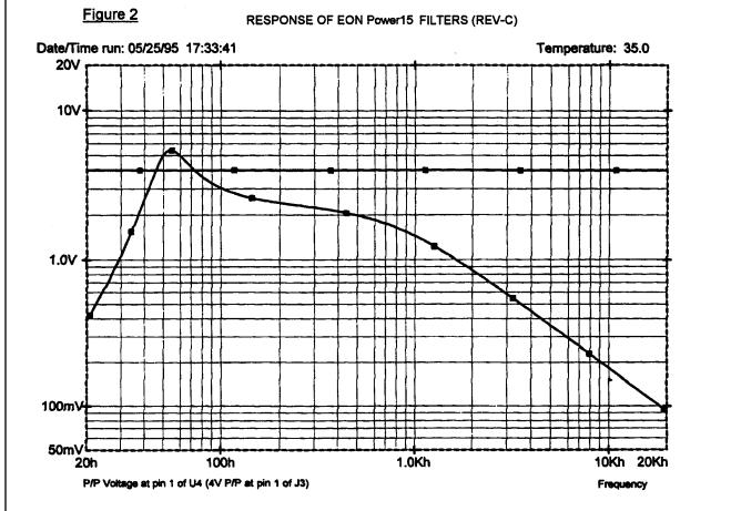
Measure the response at pin 1 of U4. Note in figure 2 above that the input voltage has not been changed. (Voltage at pin 1 of J3). The other curve represents the response at the output of the second section of the filter.
