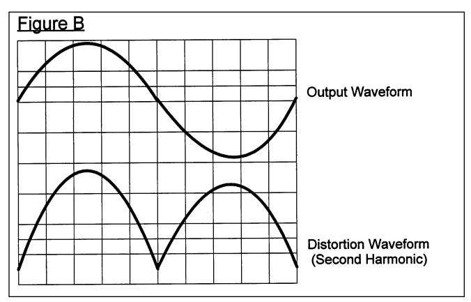
5. Excessive Second harmonic distortion in output
