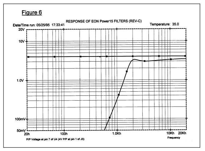
Measure the response at pin 7 of U4. Note in Figure 6 above that the input voltage has not been changed. (Voltage at pin 1 of J3). The other curve represents the response at the output of the second section of the filter.
