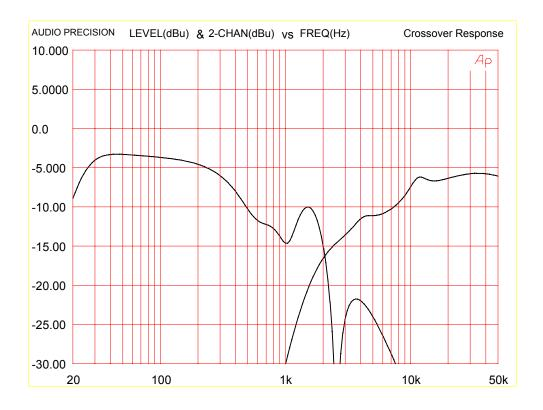
When a system under test shows a different result in the frequency response test, as shown above, using a +4dBu input signal to the XLR connector with no DIP switches selected, the source of the error can be investigated by referring to the following sections located within the troubleshooting guide.
