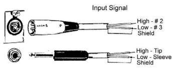
Figure 2. Unbalanced input Connections\*
