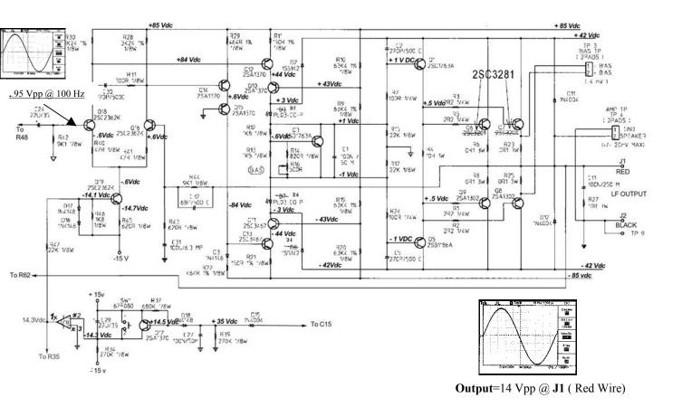
Excessive operating temperatures cause thermal switch (SW') to short activating buffer amplifier to mute the input differential amplifier and, thus, shutting down this module.
