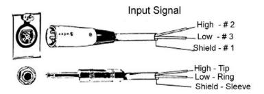
Figure 1. Balanced Input Connections\*
