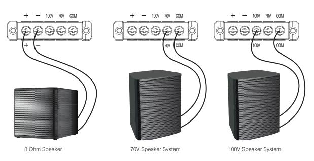
Figure 2.5.1 Output Wiring
