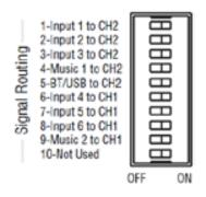
The two-channel models, VMA260 and VMA2120, include a default routing of Input channels 1-3, Music 1 and the Bluetooth/USB source to amplifier 1. Input channels 4-6 and Music 2 are routed to amplifier 2. The user may take any input and have it routed to both outputs by selecting the appropriate switch. For example, if you set switch 1 to ON, Input 1 will be routed to both AMP1 and AMP2.
