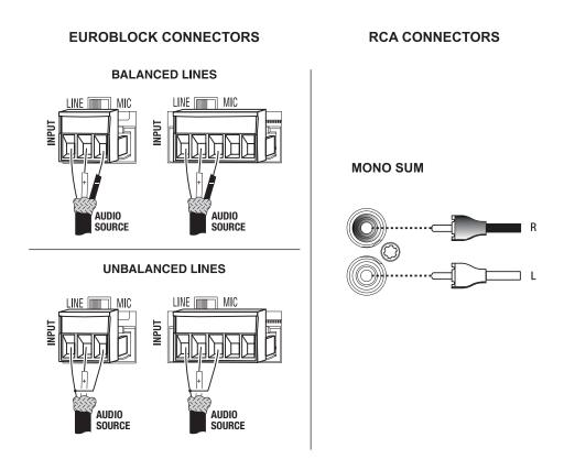
Figure 2.4.1 Input Wiring
