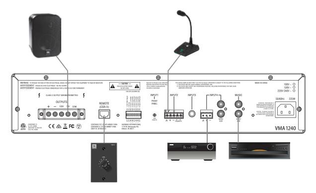
Figure 2.6.1 Wiring Audio System
