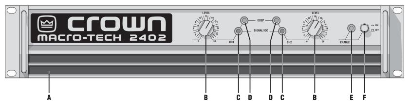
Figure 4.1 Front Panel Controls & Indicators
