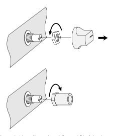
Figure 5.4 Installing a Level Control Shaft Lock
