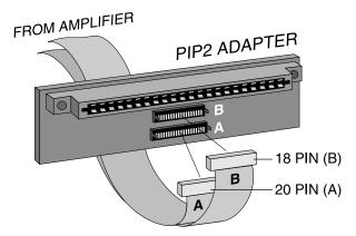
Figure 5.1 PIP2 Adapter Connection
