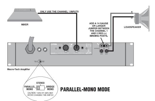
Figure 3.8 Parallel-Mono Wiring
