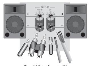
Figure 3.5 Output Connector Wiring
