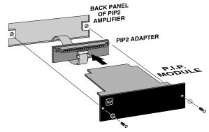
Figure 5.2 Installing a PIP Module
