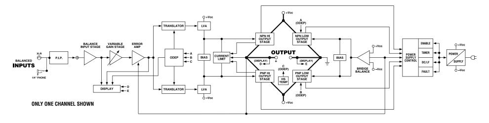
Figure 7.1 Circuit Block Diagram
