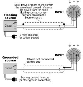
Fig. 3.8 Balanced Input Wiring
