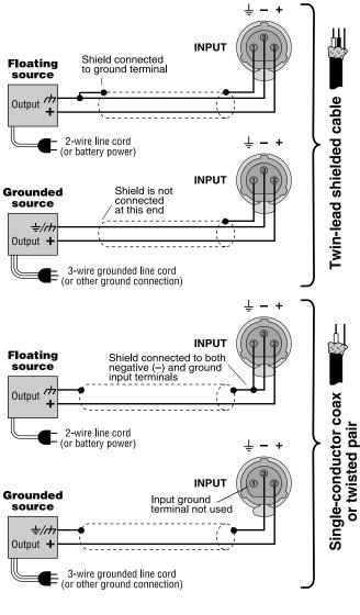
Fig. 3.7 Unbalanced Input Wiring
