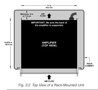
per unit. Additional air flow may be required when driving low-impedance loads at consistently high output levels. Refer to Section 7 for detailed information on thermal dissipation.
