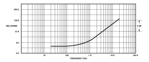
Fig. 6.5 Typical Output Impedance
