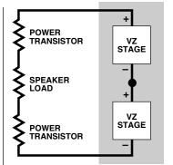
The power transistors stay cooler and are not forced to needlessly dissipate heat. This is the normal operating mode of the VZ power supply.
