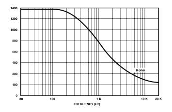
Fig. 6.4 Typical Damping Factor
