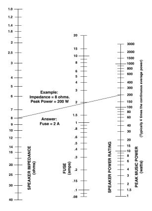
Fig. 3.13 Loudspeaker Fuse Nomograph
