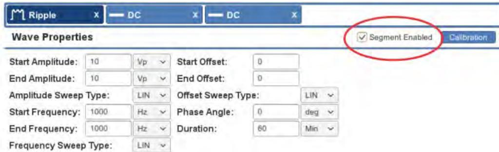
**Segment-Level Calibration:** Segments with very tight tolerances or with a calibration routine that requires levels set based on the power required to drive a non-linear device (such as MIL STD 461 or CS 101) can benefit from the new segment-level calibration function. This function allows voltage level adjustments for an individual segment within the test sequence.
