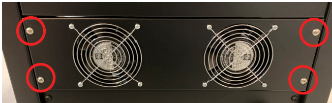
Figure 2.10 – Removing the fan panel
